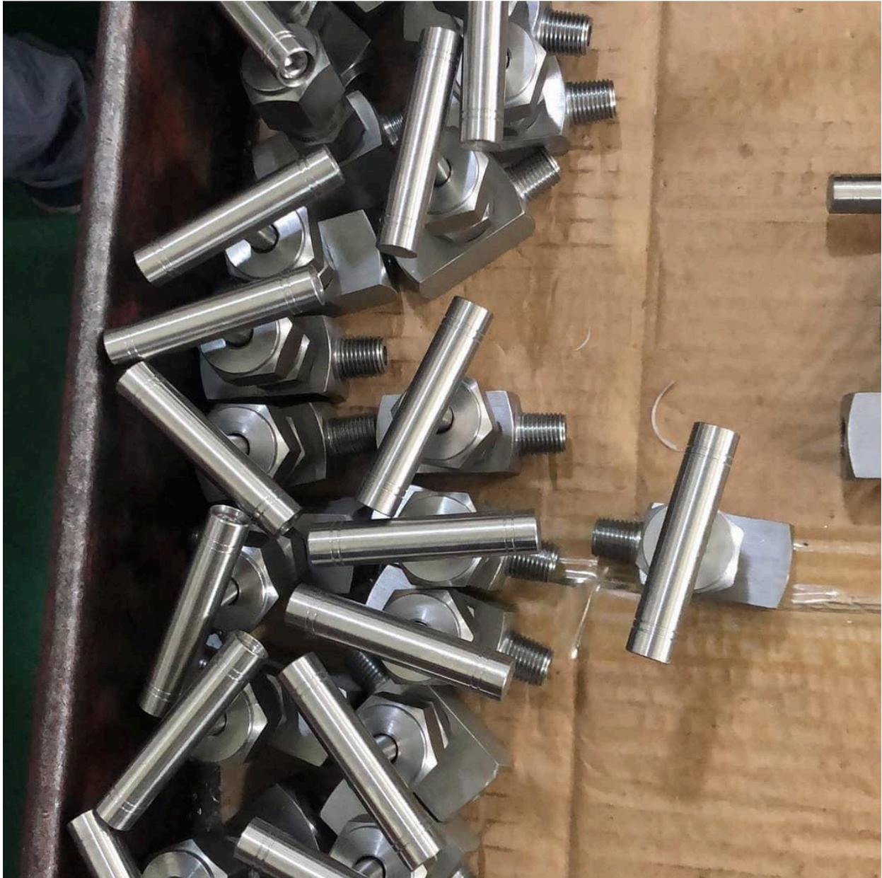
African Valve is the trusted [Needle Valve supplier in Nigeria](#). It is a type of flow control valve used to regulate the flow of a fluid through a system with very fine control and precision. It has a long, tapered point at the end of the valve stem, which is used to gradually open or close the valve seat. When the needle is fully seated, it forms a tight seal with the valve seat, preventing
